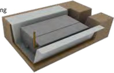
Continue with outer protection encapsulation of the geomembrane and ACO StormBrixx® system. Fold the corners of the protection fleece over-run at each end of the attenuation tank.
