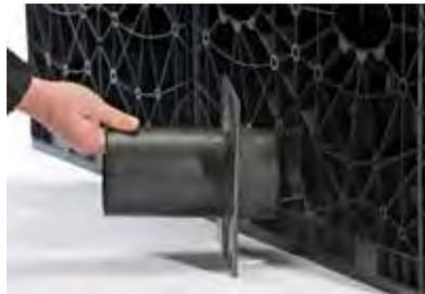
Fit connector to the side panel through holes at corners of the flange. Ensure that pipe connector is fitted so that there is adequate spigot for the joining pipe work to connect to 3" minimum (75mm).
